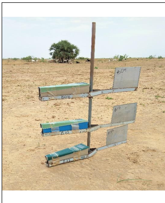
Figure 3: A Fabricated BSNE stalk loaded with sediment catchers at 5 cm, 35 cm and 55 cm height installed at the experimental site
